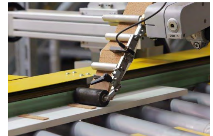
Field: Wood/ Furniture Industry Application: Lining furniture parts with cork
