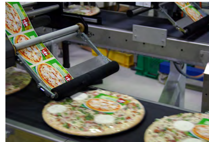
Field: Foodstuffs Application: Labelling pre-packaged pizzas
