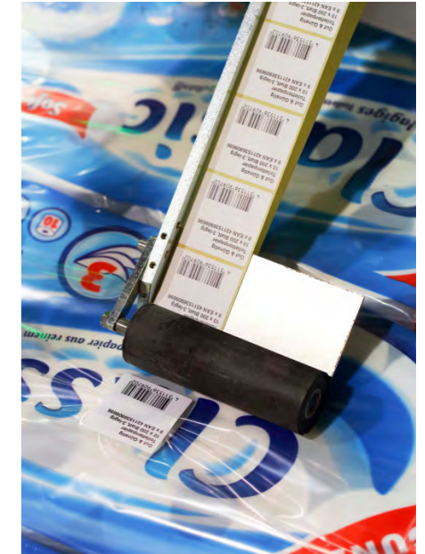
Field: Toiletries Application: Labelling toilet paper packing
